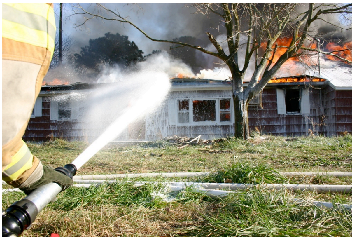
Figure 3. When confronted with a large volume of fire, applying compressed air foam through portable master stream devices has become the norm. The light-weight foam filled hose makes easy movement of the monitor to positions where the foam stream can be most effective at extinguishment.
